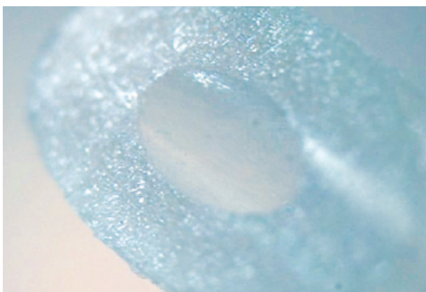
Fig 2: Draw-up needle tip, magnification of 200x
