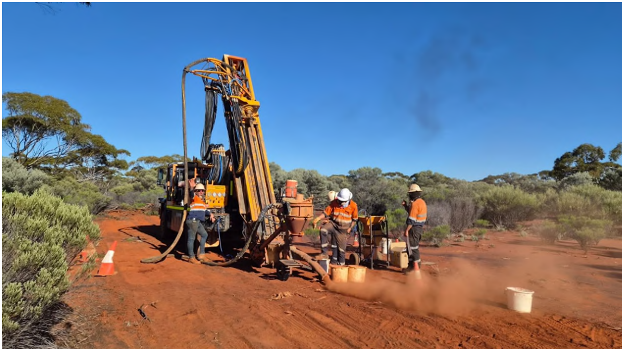
Figure 1 – Bostech Drilling's aircore drilling rig operating at the Menzies West Gold Project
