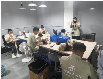
Manual Hair Stitching & Artificial Eye Installation (Source: Lingjun Onsite Visit)
