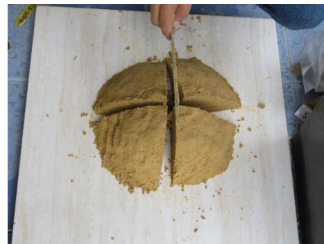
Figure 3-5 Cone and quartering of samples
