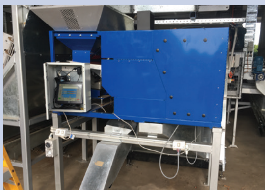
The newly installed colour sorter, which rejects any discoloured NIS, reduces the requirement for manual sorting
