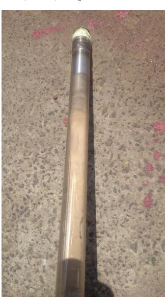
The photo is of the inlet pipe to the E-cell, shown to be plated with fine gold.
