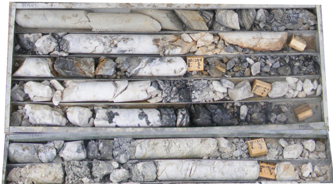
Core of hole CD15-01, Clunes, showing the character of the auriferous "structure", intersected interval 127 to 132 metres down hole.
