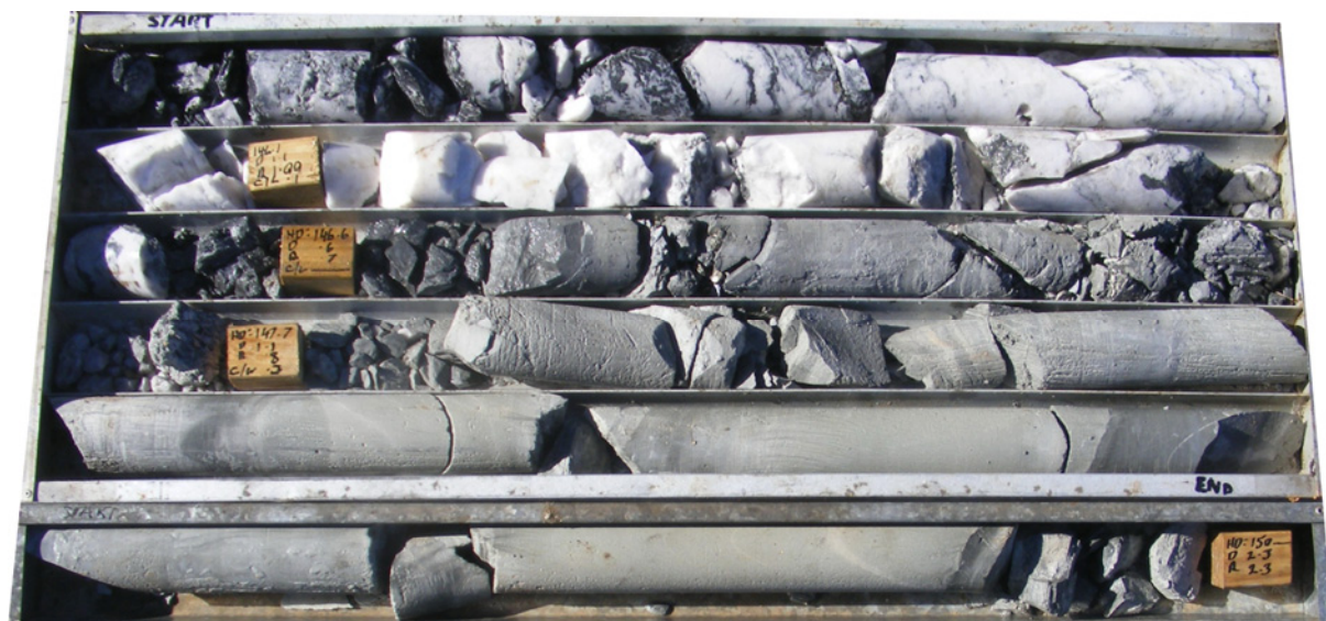
Core of Hole CD15-02, gold-rich according to assay, interval 144.5 to 148.0 metres showing state of core as-drilled.
