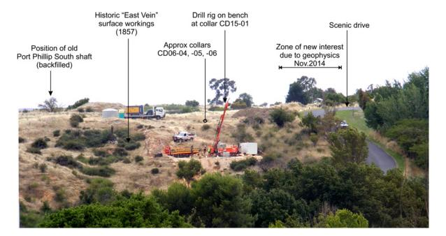
At Clunes, three (3) fully-cored holes have been diamond-drilled, off the bench in the hillside excavated for that purpose. The set-up for hole CD15-01 is as in the photograph. The other two holes were collared adjacent to hole one, on the bench.
