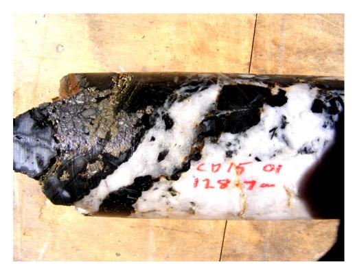
These first 3 holes this year have indeed passed through four readily observed quartz structures. Two of these evident quartz structures are about the expected historic positions of named veins - those named as "East Vein", and the "Old Man Vein", about which much is written.
