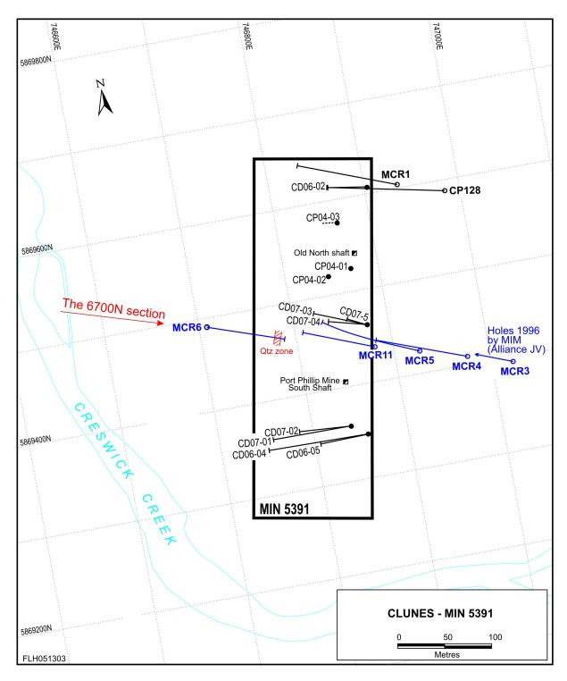
At Clunes, a program of R.C. drilling (M.I.M Exploration Pty Ltd) with some diamond drilling (as tails to deepen 4 of the RC holes) all took place in the first quarter, year 1996. A total of 18 holes were drilled at a total reported cost of \$518,703 (1996 dollars) of which \$241, 735 was paid to drilling contractors.
