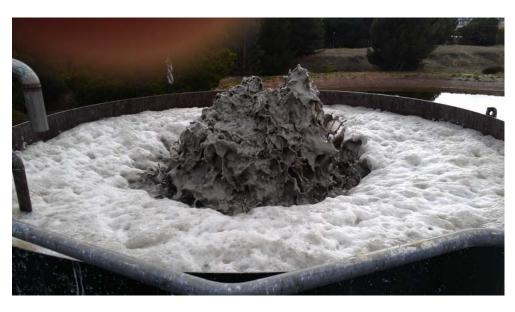
On discharge from a pachuca, the aerated sands do consolidate rapidly. Substantial settlement is achievable within 24 hours. This should ensure good environmental control at site.
