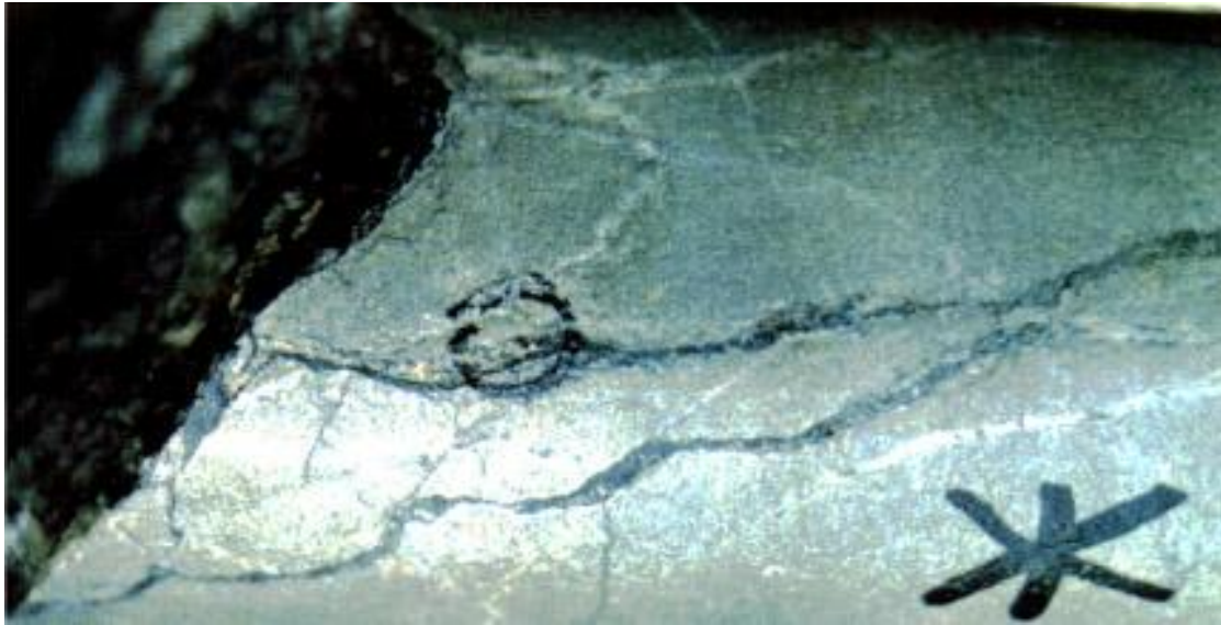
Plate 2. Photograph of drill core from MDD-001. Note presence of visible gold within a low amplitude, black graphite-chlorite-pyrite stylolite seam, within sericite altered, hydrofractured sandstone. (Assay 75-76m: 12.0 g/t Au).
