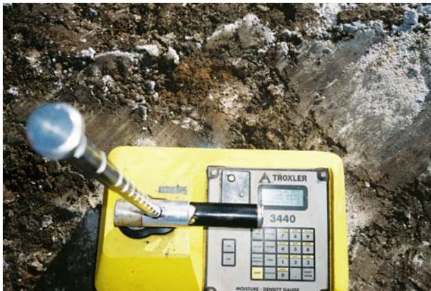
This is the "face" of the yellow box-mounted equipment seen in the photo above. It assists in Density Determination. It is a Nuclear Density/Moisture Gauge.
