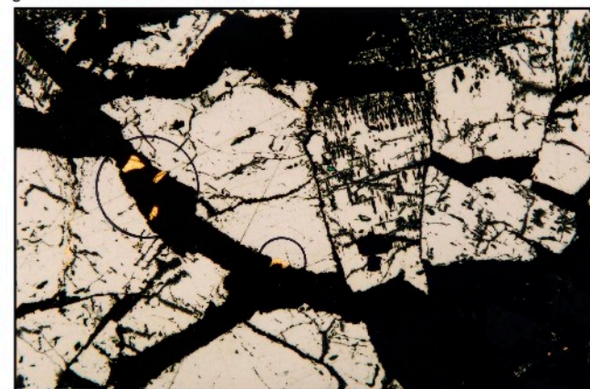
CD06-2 at depth 118m Original area covered by the micro-photo size - 0.6mm x 0.4mm Four gold grains up to 20 micron size, here within a quartz veinlet between arsenopyrite
