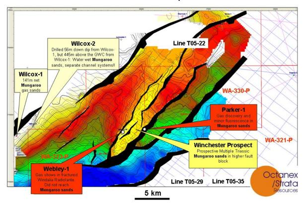
In summary, the joint venture are undertaking the OBC 3D seismic survey in order to visualise the structure and stratigraphy of the feature, which may provide a sizeable and attractive drilling target.
