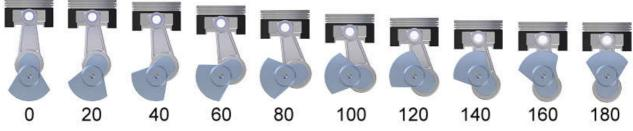
Degrees of Rotation on a Power Stroke
