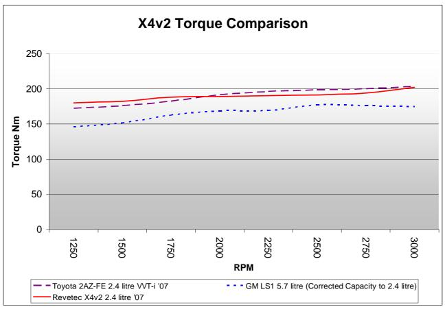
Even though we are not using VLIP, VVT and 4 valves per cylinder, we have achieved:
