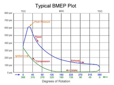
right angles to the crankshaft. If we look at a typical Brake Mean Effective Pressure (BMEP) plot at lower RPM you will notice that the peak cylinder pressure is around 30 degrees ATDC.
