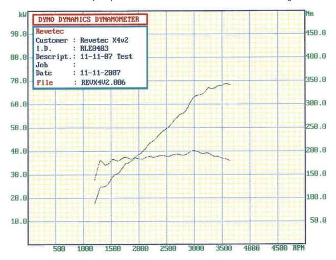
Note: We have achieved a torque figure of 180Nm@1,300rpm.
