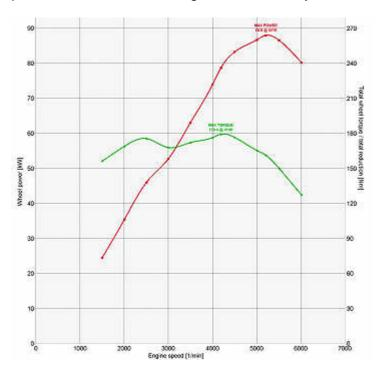
The Variable Length Intake Ports on this engine dyno graph of the Toyota system clearly shows the effect of this feature in the torque curve (In green).
