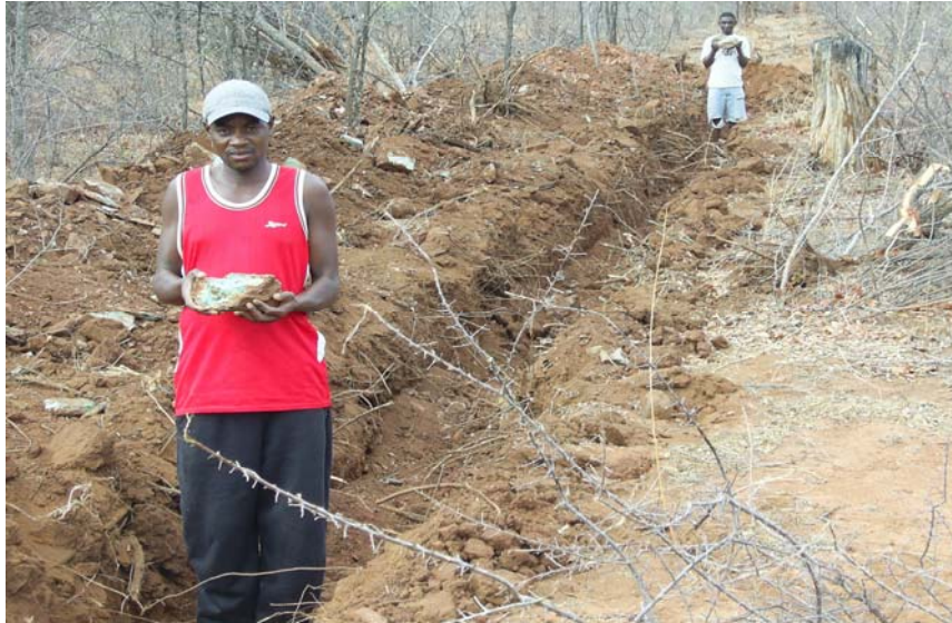
Photograph 1: trench with visible copper mineralisation from Airstrip Copper Prospect
