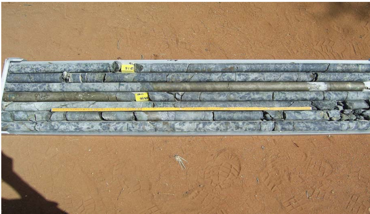
Photograph 3: photograph of drill cores from drill hole MAI-05_23 showing 1.28 metres of massive sulphides from 94.14 m to 95.42 m downhole
