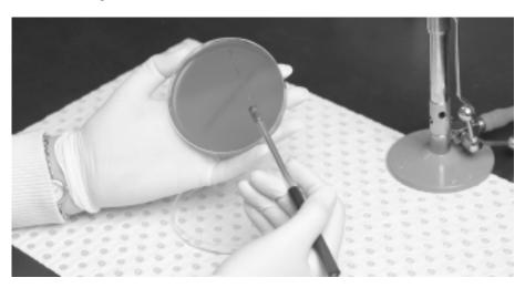
The core MicroStreak® technology allows automation of Agar Plate Inoculation and streaking. The Company proposes to incorporate the technology into an instrumentation system to automate manual processes associated with routine Agar Plate preparation.
